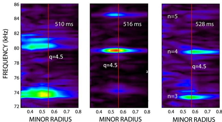
FIG. 3 (color online). Radial profiles of  $\delta T_e/T_e$  frequency (in lab frame) spectra (in arbitrary unit) measured in the DIII-D experiment at  $t = 510$  ms, 516 ms, and 528 ms, respectively. The vertical red lines indicate the location of the  $q = 4.5$  flux surface at different times.
