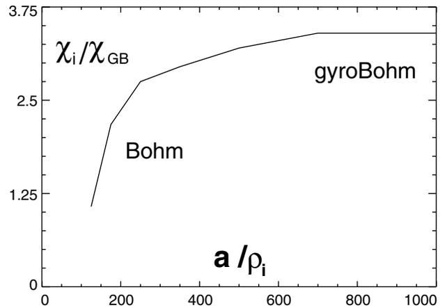
FIG. 3. Ion heat conductivity vs tokamak minor radius.
