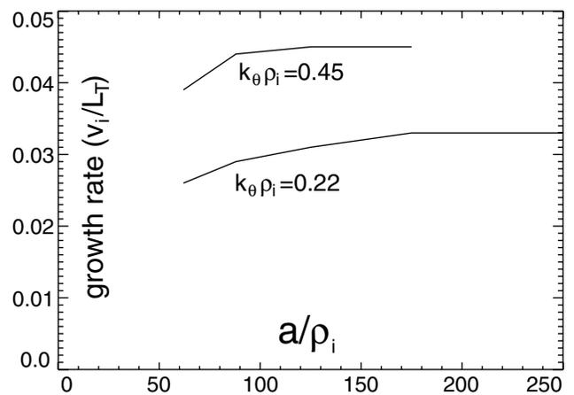
FIG. 4. Linear growth rate vs device size.
