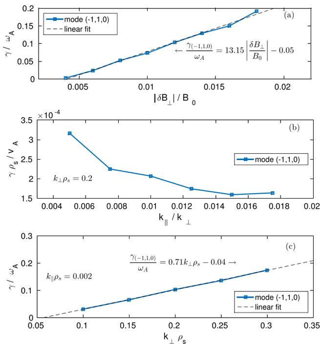
FIG. 5. Growth rates  $\gamma/\omega_A$  of mode  $(-1, 1, 0)$  with respect to the pump wave (a) amplitude  $\delta B_{\perp}/B_0$ , (b) parallel wavenumber  $k_{\parallel}$ , and (c) perpendicular wavenumber  $k_{\perp}$ .
