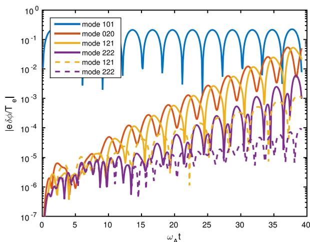
FIG. 2. Time history of the scalar potential  $\delta\phi$  of the pump wave 101 and daughter waves. Solid lines represent the simulation in which mode 101, 020, 121, and 222 are kept; while dash lines represent the simulation in which mode 101, 121, and 222 are kept.
