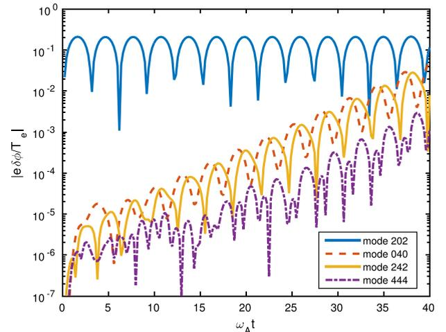
FIG. 1. Time history of scalar potential  $\delta \phi$  of the pump wave 202 and daughter waves with the highest amplitudes in the simulation keeping all daughter waves.
